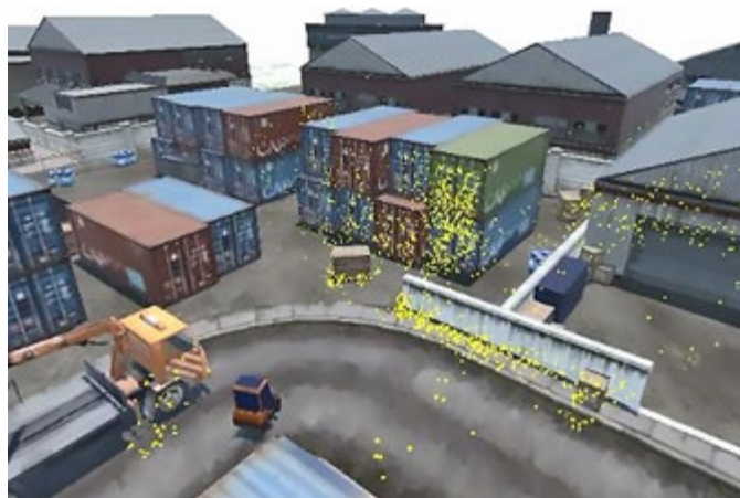
The SLAM evaluation framework showing the algorithm's point cloud representation of the scene, corresponding to the location of objects and surfaces observed as the vehicle drives around a simulated industrial scene
