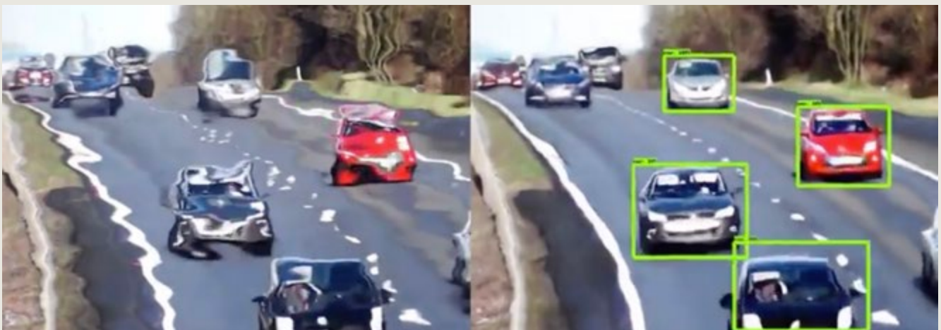
SharpWave™ can remove the effects of distortion (left image) to drastically improve the performance of object detection and classification of vehicles (right image)
