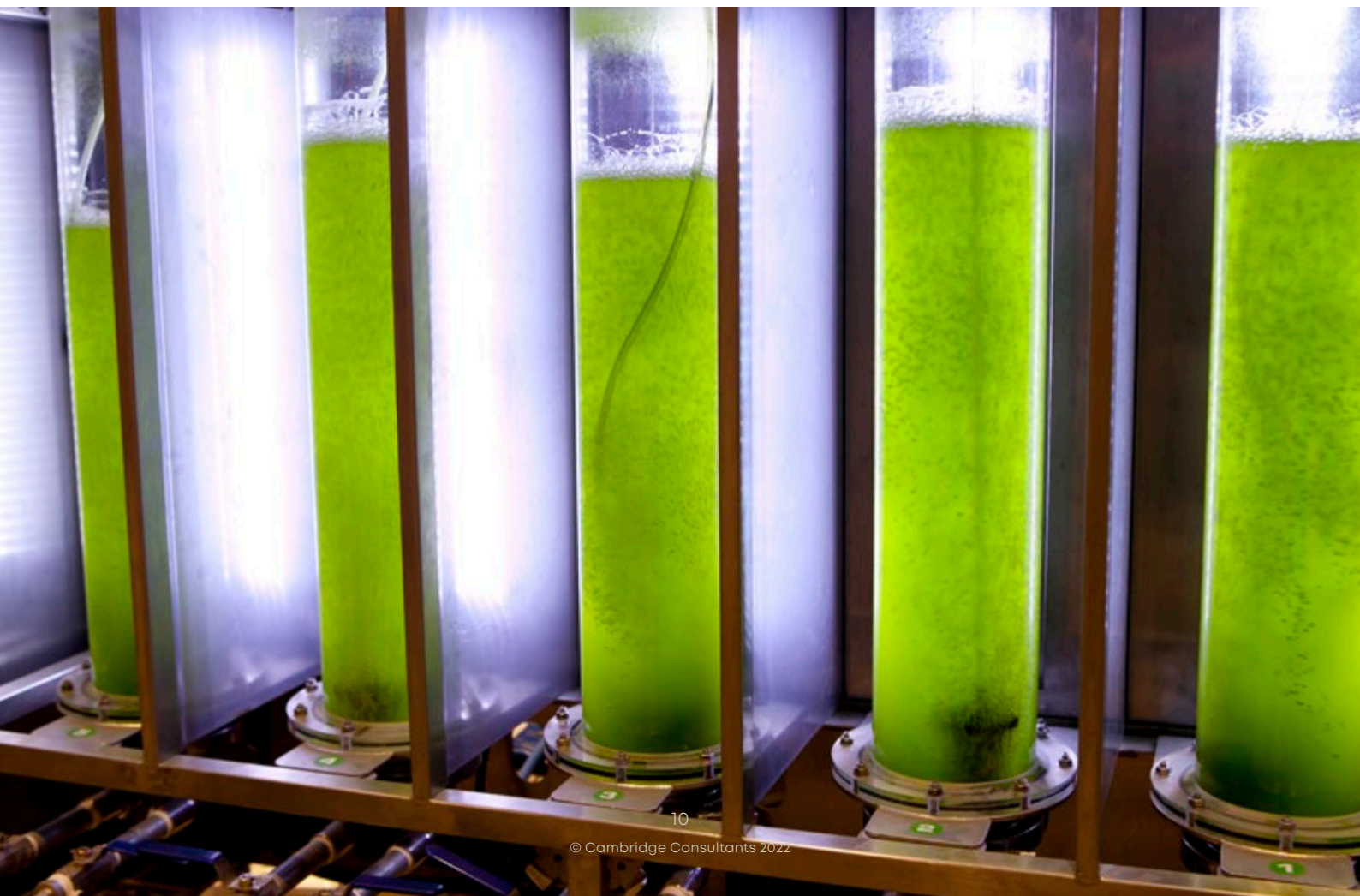
Image 2: A photobioreactor - a bioreactor that utilizes a light source to cultivate phototrophic microorganisms
