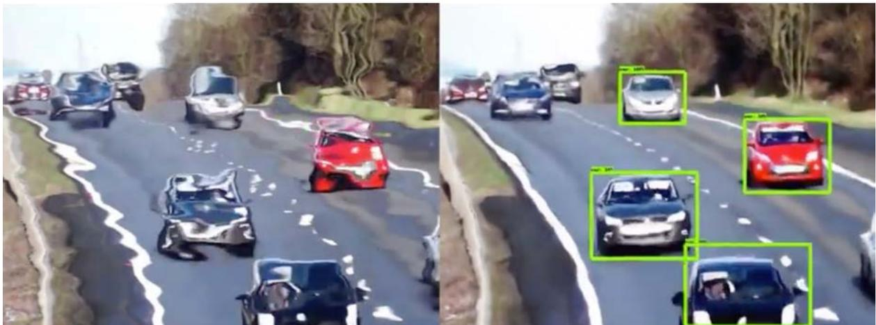
DeepRay can remove the effects of distortion (left image) to drastically improve the performance of object detection and classification of vehicles (right image)
