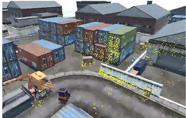
The SLAM evaluation framework showing the algorithm's point cloud representation of the scene, corresponding to the location of objects and surfaces observed as the vehicle drives around a simulated industrial scene
