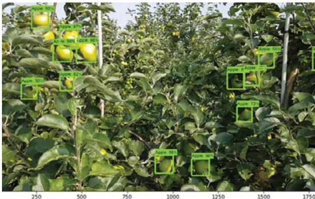
FIGURE 5: Fruit detection in a natural environment, utilizing footage from a cheap camera and machine learning.
